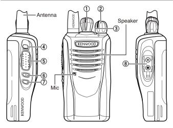
① **Channel Selector** Rotate to select a channel.
