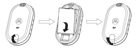
Note: The CLP Series radios standard packaged models come with standard Lithium Ion battery and the standard Lithium Ion battery door. For option, customers can order Hi-capacity Lithium Ion battery (P/N HKNN4013) and the Hi-capacity Lithium Ion battery door (P/N HKLN4440).
