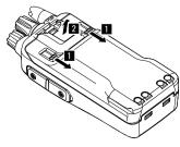
Detaching: Lift the tab up (1), and slide the belt clip in the direction of the arrow (2).
