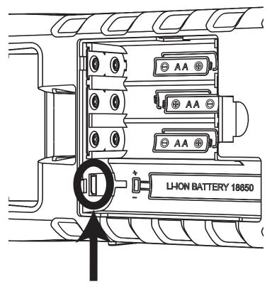
Connect the BATT26L Li-ion battery here.
