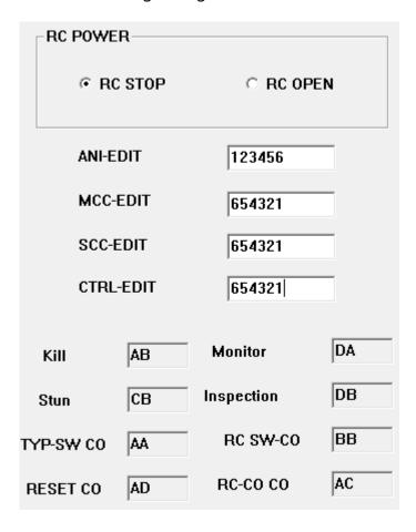
The RC POWER section determines if the radio will allow a remote power on/off request.
