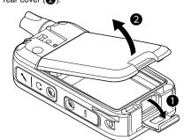
2. Install the supplied battery pack so that the terminals of the battery pack and the transceiver meet.
