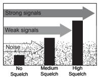
While listening to a channel, adjust the **SQUELCH** knob until the noise is filtered and you can hear only the transmission. If you switch to a channel with a lot of noise or a weak transmission, you may need to readjust the squelch level again.
