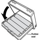
the battery case, check the rubber seal. Make sure the seal is seated in the groove and there is no dirt or debris on it. If the rubber seal looks worn or damaged, contact customer service to order a replacement (see back cover for contact information).
