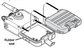
**Note:** Each time you remove the battery, check the rubber seal around the battery compartment. Make sure the rubber seal is seated in the groove and there is no dirt or debris on it. If the seal looks worn or damaged, contact customer service to order a
