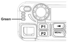
**NOTE**: The green LED lights up while the radio is transmitting and blinks rapidly when the radio is receiving a privacy-enabled call.
