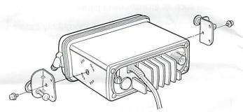
⑤ Tighten the locking nuts (rotate counterclockwise) so that the MB-45 is securely mounted in position as below.
