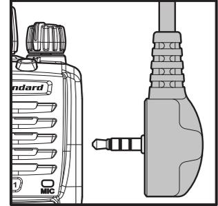
*Note 1): Save the original plastic cap and its mounting screws. They should be reinstalled when not using the Speaker/Microphone.*
