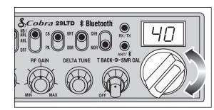
• Select O one of forty channels and adjust volume. The selected channel is indicated by the LED readout directly above the channel selector knob
