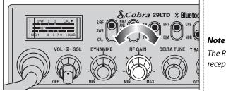
Rotate the RF Gain knob counterclockwise to reduce gain in strong signal areas. In weak signal areas turn clockwise to increase gain. External Speaker
