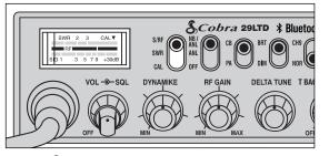
The S/RF-SWR-CAL switch must be in the S/RF position.
