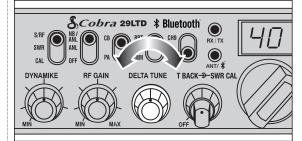
**1** *Rotate* O Delta-Tune knob to the center position for optimum tuning.
