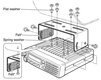
When using self-tapping screws
