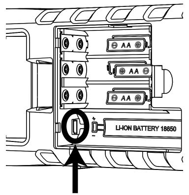
Connect the BATT20L Li-ion battery here.
