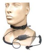
Medium duty throat mic with Kevlar™ cabling, in-line PTT with optional finger PTT jack, crystal clear audio tx/rx, multiadjustable elastic throat band and 7 interchangeable ear options. Optional remote finger PTT available.
