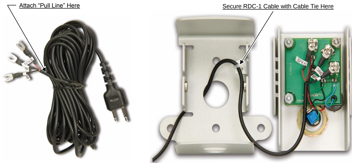
Figure-3: RDC-1 Installation
